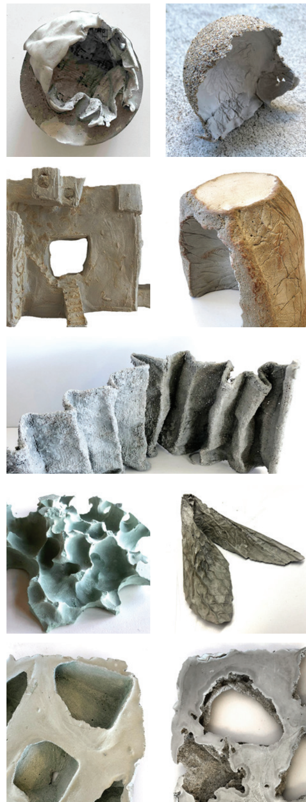
Fig. 14-22 Selection of early studies from creative casting with sustainable formwork: biofoam, bioplastics, canvas, clay, paper, and sand. Clockwise from top right: A. Nikzad, S. Park, W. Wong, D. Dinh, A. Nguyen, A. Nguyen, J. Velasco, J. Lindberg.
