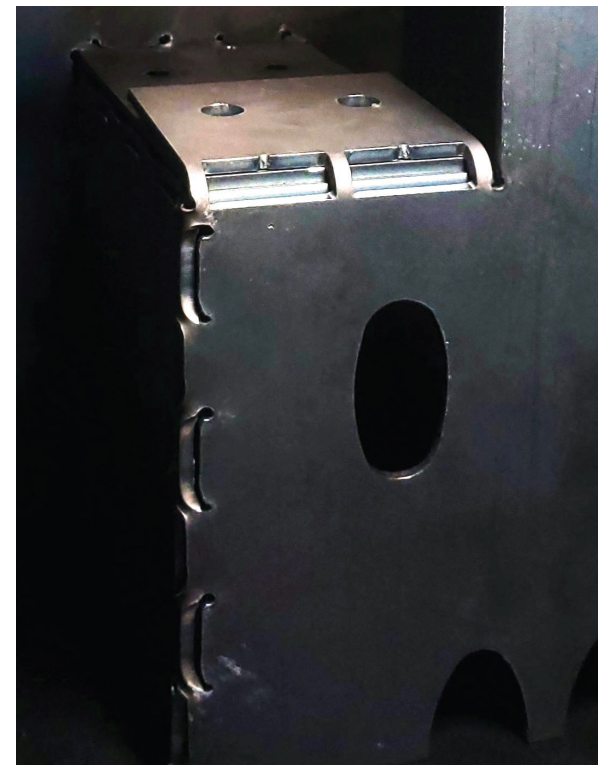
Fig. 9 Final detail iteration before adding to full sheet pattern from Flat Force Fold Form research studio Fall 2021 by Paul Monson
