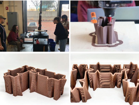
Fig. 5 The image at the top left shows a student group 3D printing a clay block. The image at the top right is an up-close photo of the printer printing. The images on the bottom row show the blocks and how they tessellate.
