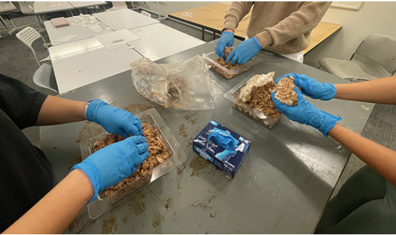
Fig. 4 Regrinding and packing forms with mycelium and hemp mixture. Student Work.
