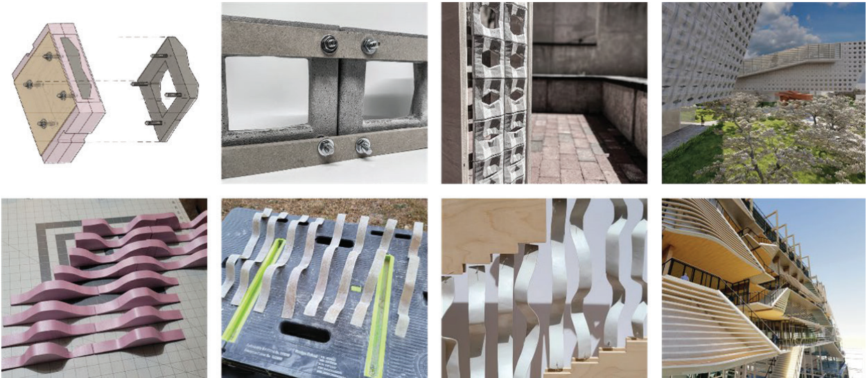
Fig. 6 The images on the top row show a student project that focused on 2-part CNC milled formwork to create custom tiles with variable opening sizes to control daylighting. The aperture sizes were informed by computational analysis of daylighting. The bottom row of images shows a project that utilized robotic hot wire cut foam as a mold for fiberglass louvers.
