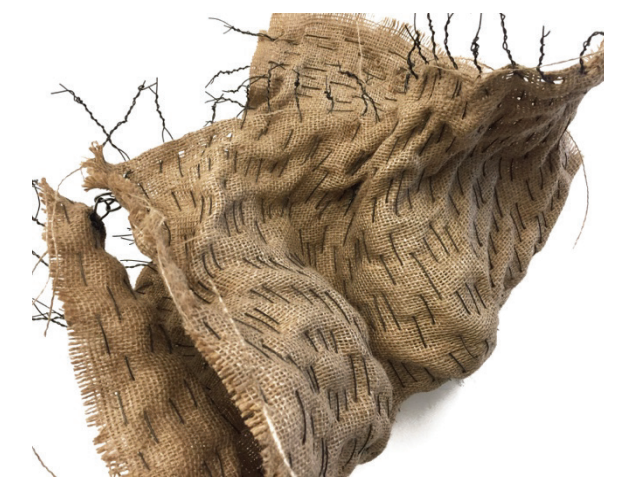
Fig. 8 Formable and reformable, malleable hessian textile interwoven with copper wire, L. Lawrence, 2019
