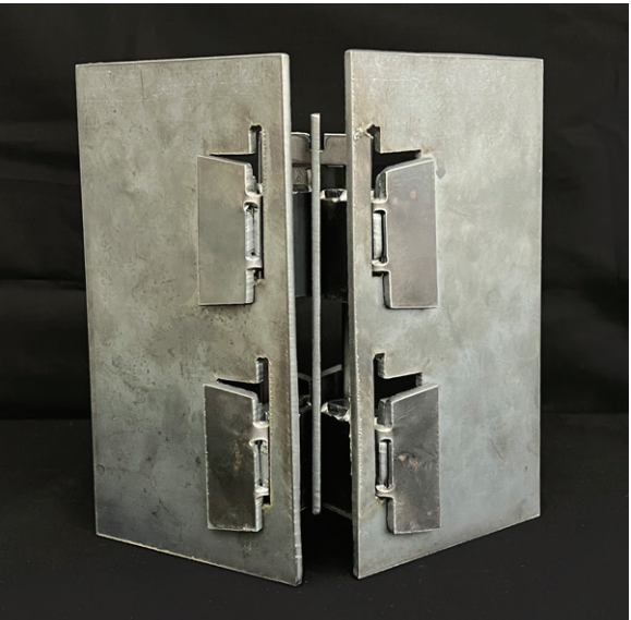
Fig. 10 Demountable corner connection from the initial offering of ARCH 715 Metal Fabrication for Architecture at Kansas State University, Fall 2020 by Katherine Duloheery.
